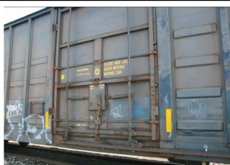
Typical plug door. This door pops out on rotary hinges then rolls down runner tracks. See the hinge and runner track just below.
