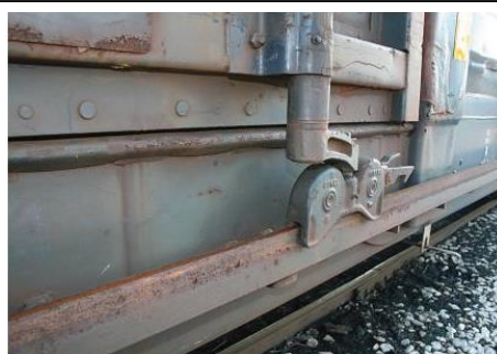
Typical plug door. This door pops out on rotary hinges then rolls down runner tracks. See the hinge and runner track just below.
